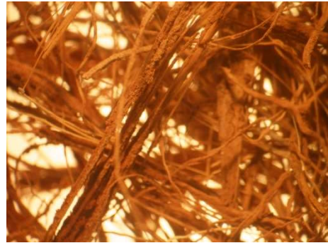
Fibers treated with 0.172% of Ca(OH) 2 .
