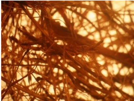
Fibers treated with 2% of NaOH.
