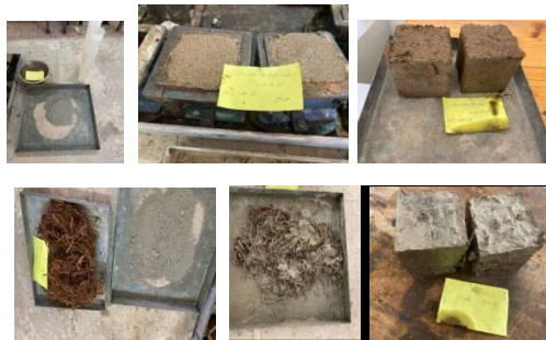
Figure 4: prepared date palm fiber (remaining on sieve 0.6 mm) reinforced mortar introduced as percentage of cemen weight.
